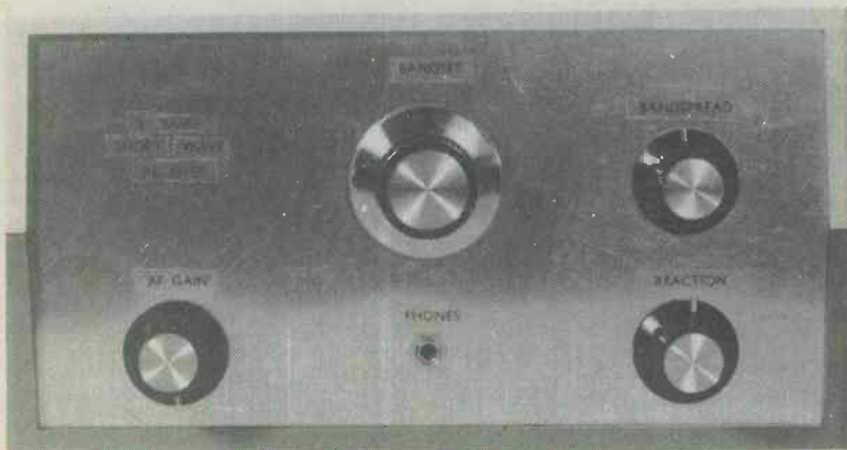
The 3 band short wave receiver is housed in a ready-made Verobox. The controls are well spaced out for ease of operation
